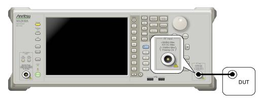
Figure 2.2-1 Signal path setup example
